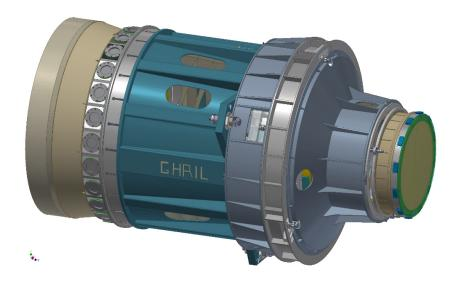
The Central Can (already manufactured) is attached to the vanes which are attached to the Focus Translation System. In this photo the dummy PFC is inserted into the Central Can.
