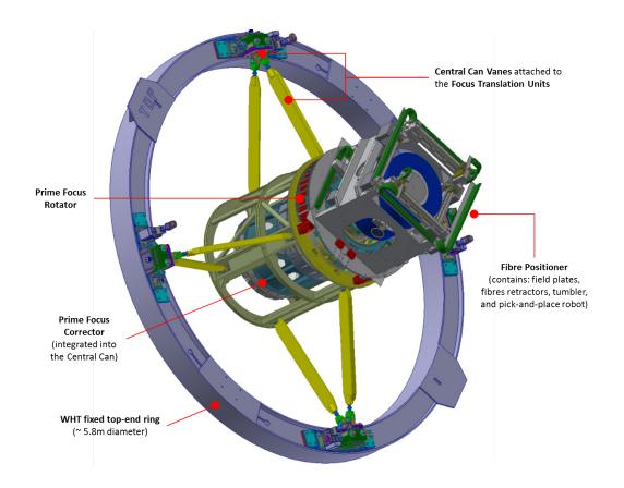
The purpose of the WEAVE Prime Focus Corrector is to correct for the optical aberrations in the two-degree field-of-view. The corrector also includes an Atmospheric Dispersion Corrector (ADC) which consists of two pairs of counter-rotating, air-separated doublets, to compensate for atmospheric dispersion whilst the telescope is moving in elevation.
